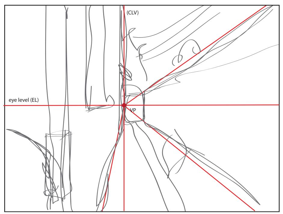
Measure the angles of the walls and any other large masses in the space, such as fences in this example. Remember that all parallel lines converge to the same VP. If your angle measurements are not converging to the same point you have either made a mistake when measuring or a mistake in finding the accurate EL and CLV, or possibly both. Be patient, careful and re-check all of your measurements.
