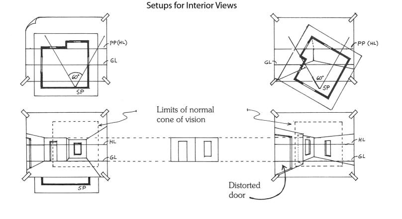
Here again, areas that extend beyond the cone of vision may be included if there are no objects of furniture to make the distortion obvious. Notice above how the door stretches to the left. Often, interior views are rendered in such a way that the walls are allowed to fade out—an effect similar to that experienced in our peripheral vision.
