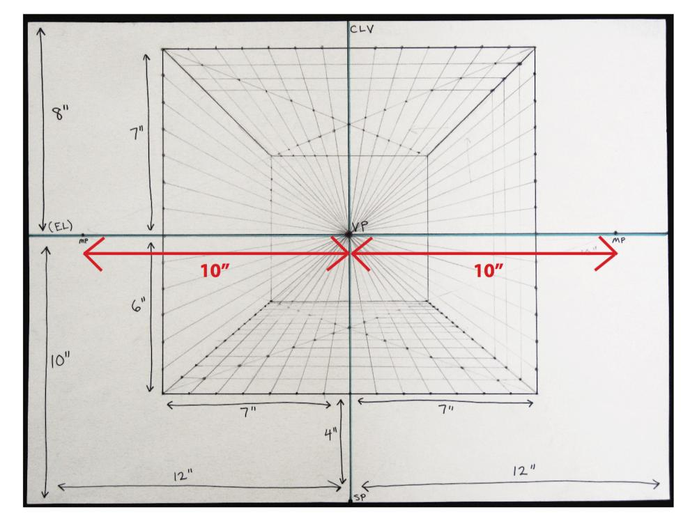
**Measuring Point Example (MP)** - Reminder: To find the measuring points, simply measure 10" over from the VP. (This is the same distance as the VP to the SP)
